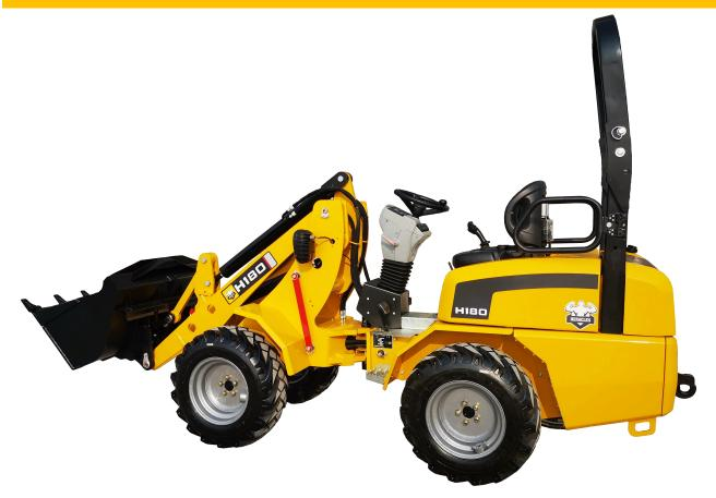
Thanks to compact dimensions and excellent control, Heracles Wheel Loaders cannot only work in manay grounds, but also tackle different problemss. The hydraulic drive system makes operation more comfortable and easier. Operators can learn how to use the machines much more quickly. The individual wheel motor gives an excellent ground clearance that can make machines to be operated in restricted areas. Reliability, durability and low maintenance makes wheel loaders a good investment.
