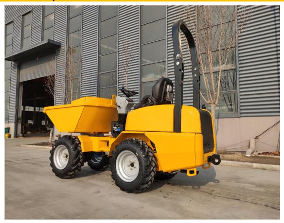
Thanks to compact dimensions and excellent control, Heracels Wheel Dumpers cannot only work in manay grounds, but also tackle different problemss. The hydraulic drive system makes operation more comfortable and easier. Operators can learn how to use the machines much more quickly. The individual wheel motor gives an excellent ground clearance that can make machines to be operated in restricted areas. Reliability, durability and low maintenance makes wheel dumpers a good investment.
